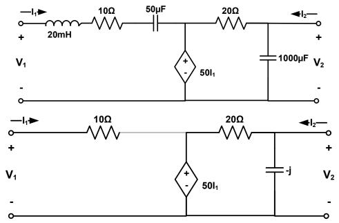
$V_1 = h_{11}I_1 + h_{12}V_2$  $I_2 = h_{21}I_1 + h_{22}V_2$
